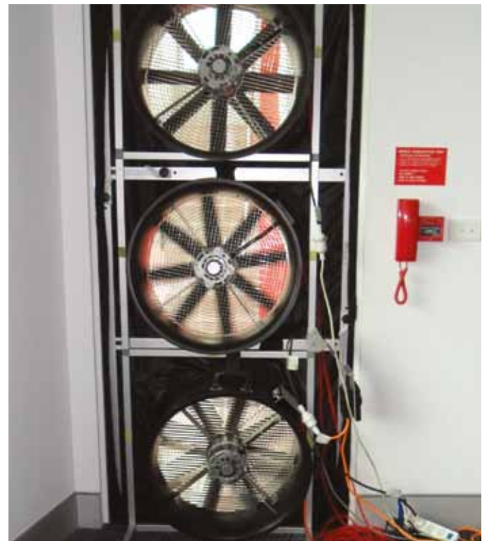
Figure 2: Blower door used for air leakage testing.
